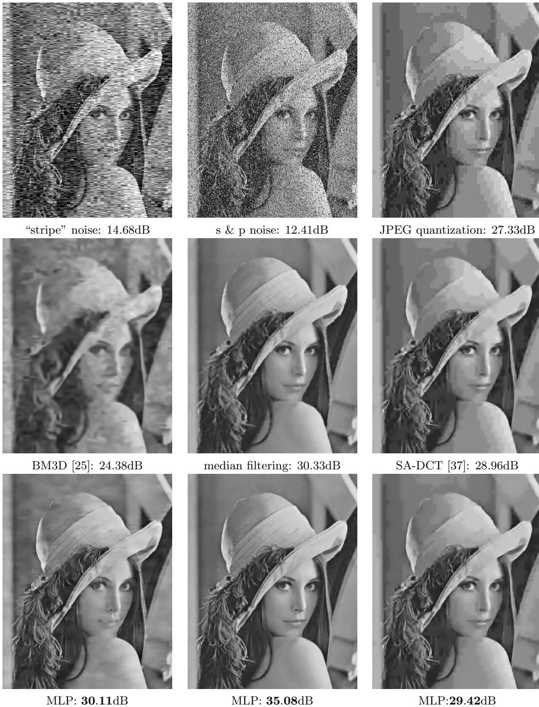
Figure 5.15: Comparison of our method to other on stripe noise (left), salt-and-pepper noise (middle) and JPEG quantization artifacts (right). BM3D is not designed for stripe noise.
