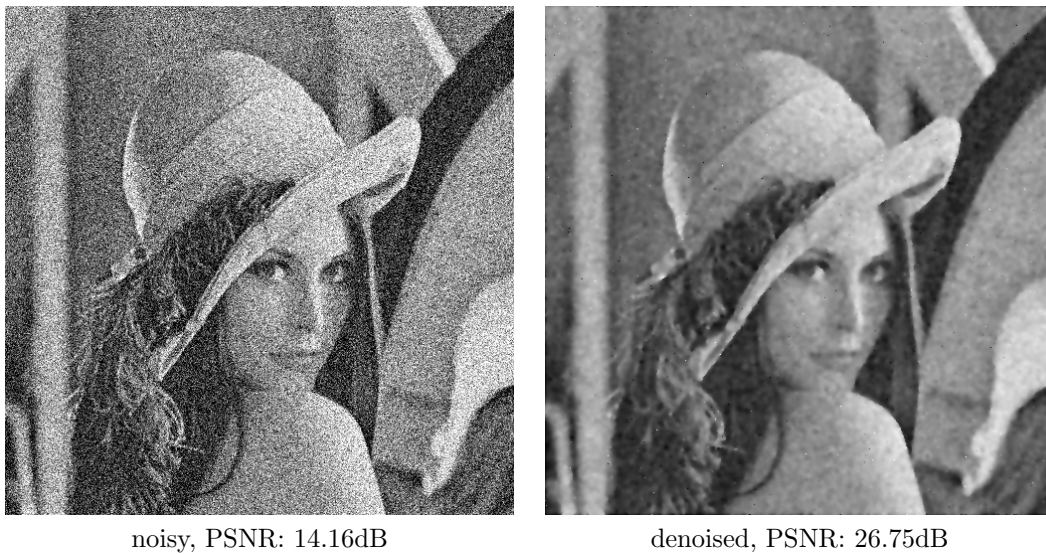
Figure 2.8: Results using anisotropic diffusion. We used \kappa = 40 , 12 iterations and c(\nabla I) = (1 + (\frac{\nabla I}{\kappa})^2)^{-1}
