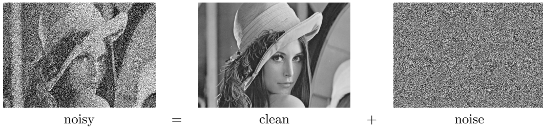
Figure 1.1: A noisy image is assumed to be the sum of an underlying clean image and noise.
