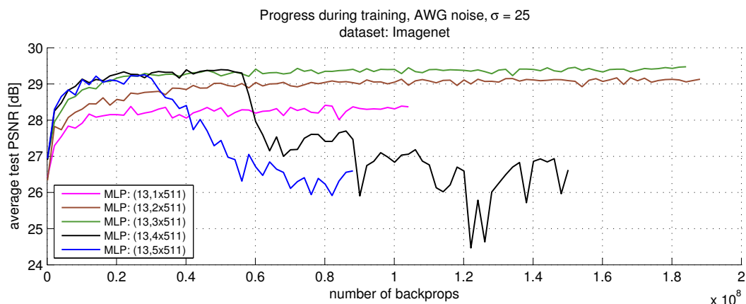
Figure 6.3: More hidden layers usually help. Too many hidden layers with few hidden units cause a catastrophic degradation in performance.
