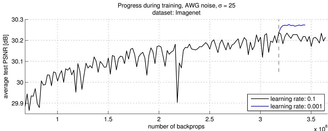
Figure 9: Fine-tuning improves results and reduces fluctuations in the test error. The vertical dashed line indicates where the learning rate was switched from 0.1 to 0.001. The two curves therefore only disagree starting at the dashed vertical line.
