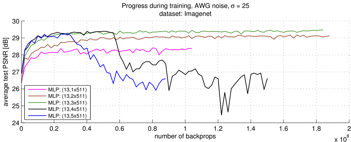
Figure 3: More hidden layers usually help. Too many hidden layers with few hidden units cause a catastrophic degradation in performance.
