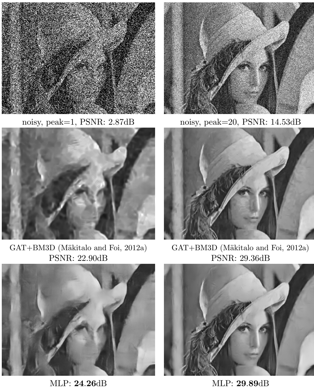
Figure 11: Comparison of our method to GAT+BM3D (Mäkitalo and Foi, 2012a) on images corrupted with mixed Poisson-Gaussian noise, which occurs in photon-limited imaging.
