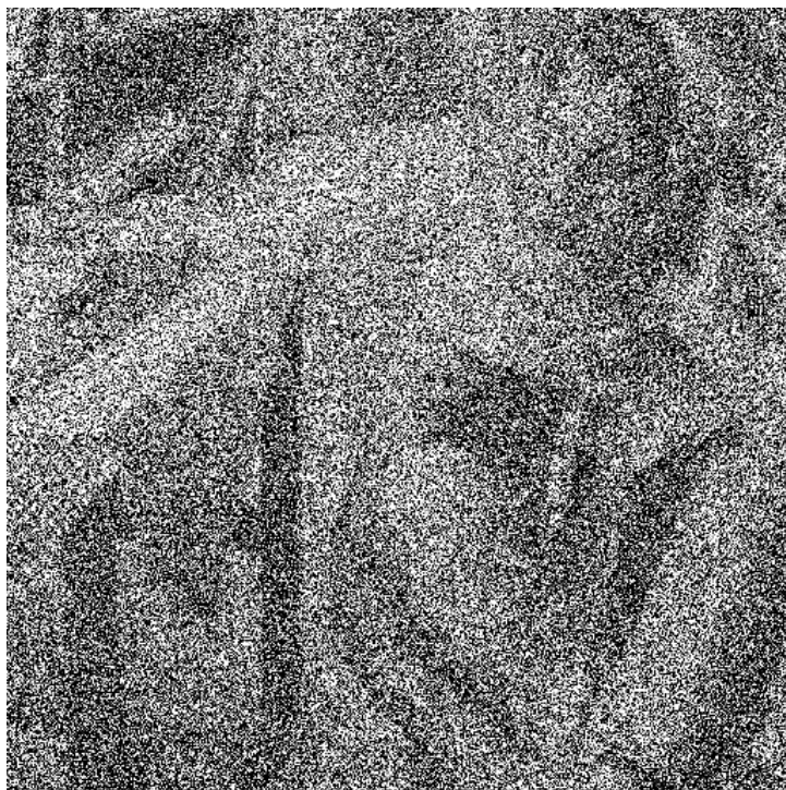
noisy \sigma = 200 PSNR: 7.59dB, SSIM: 0.074
